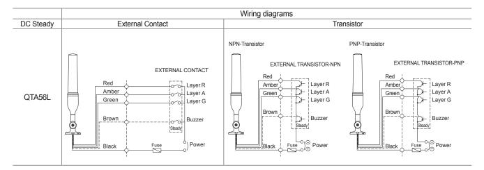
• External power line/ External signal line - UL1007 AWG22(0.3sq) 400mm
