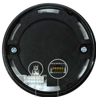
Lever for sound adjustment Channel switch
