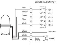
• External power line - UL1015 AWG18(0.75sq) x 2C 400mm External signal line - UL1007 AWG22(0.3sq) 400mm
